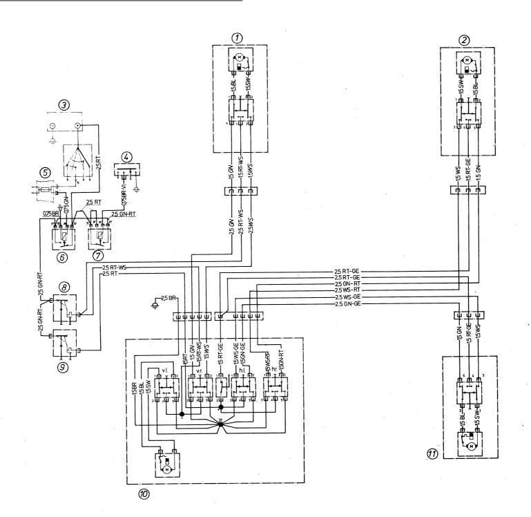
E3 / E9 - elelktrisch verstellbare Aussenspiegel - electric controlled ext. rear view mirror
