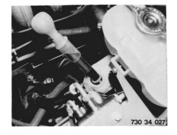
Remove instrument panel trim at bottom left - see 51 45 180. Lift out bayonet clip (1) and remove pin (2) on piston rod.
